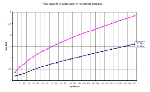
The two slopes represent the upper and lower flows that are currently used in Western and Northern Europe for dimensioning of flow demand in residential buildings. By striving to make dimensions closer to the lower line in Figure 4 above, one can obtain better economical and maintenance results for both substations, network and production. See chapter 2.7.2.
