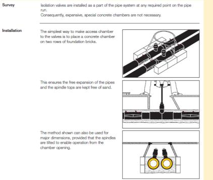
Example of pre-insulated valves buried directly in the ground with access from street level.
